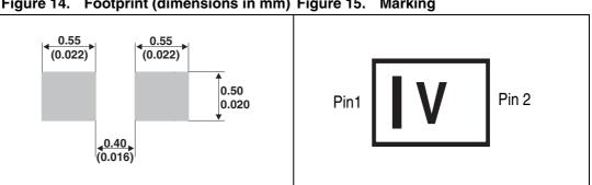
Figure 14. Footprint (dimensions in mm) Figure 15. Marking
