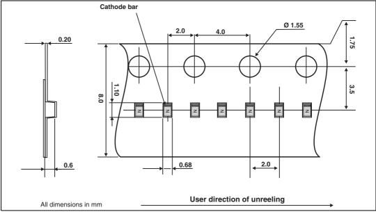
Figure 16. Tape and reel specifications
