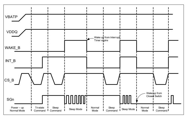
Figure 17. Low-power mode to Normal mode operation
