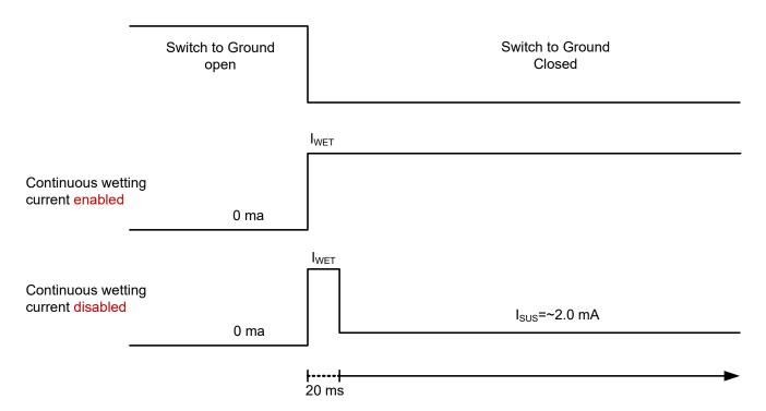
Figure 25. Pulsed/continuous wetting current configuration
