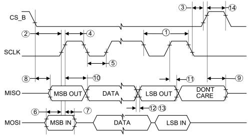
Figure 7. SPI timing diagram
