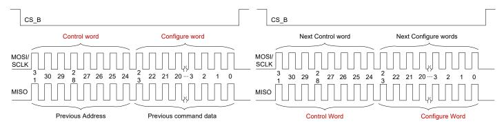
Figure 22. SPI write operation
