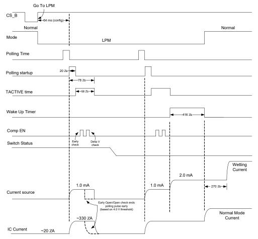
Figure 16. Low-power mode typical timing
