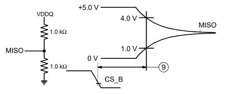
Figure 8. MISO loading for disable time measurement
