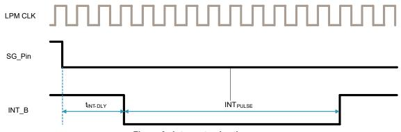
Figure 6. Interrupt pulse timer
