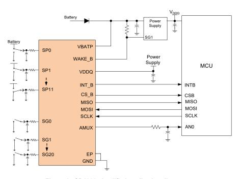
Figure 1. CD1030 simplified application diagram
