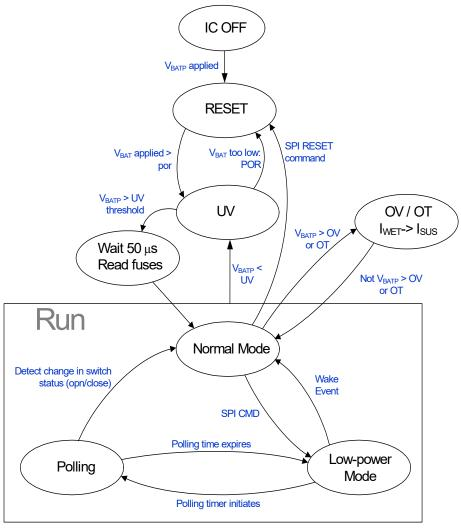
Figure 18. CD1030 state diagram
