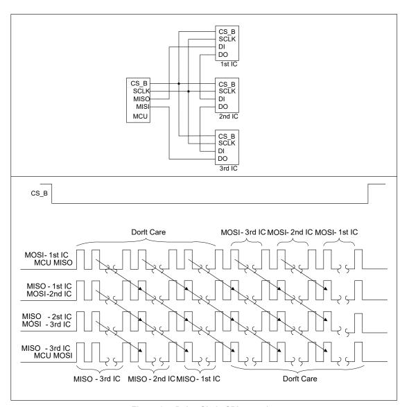
Figure 24. Daisy Chain SPI operation
