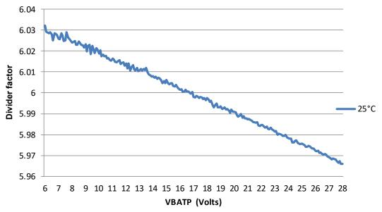
Figure 4. Divide by 6 coefficient accuracy
