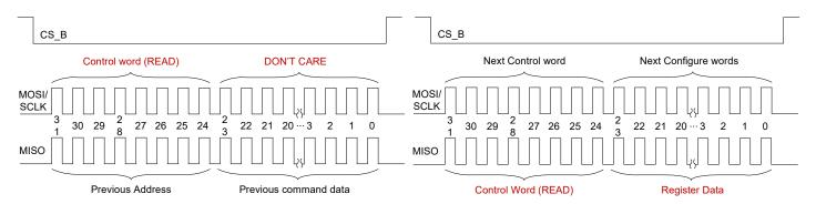
Figure 23. SPI read operation
