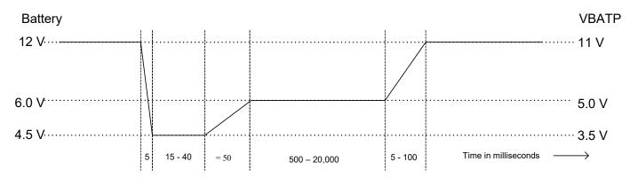
Figure 14. Battery crank profile
