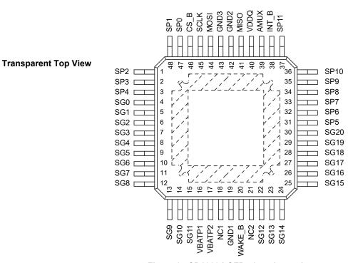
Figure 3. CD1030 LQFP-48 package pinout
