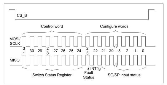
Figure 21. First SPI operation (After POR)
