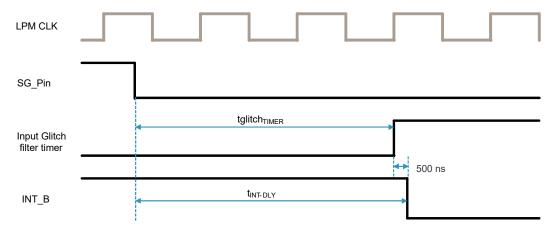
Figure 5. Glitch filter and interrupt delay timers
