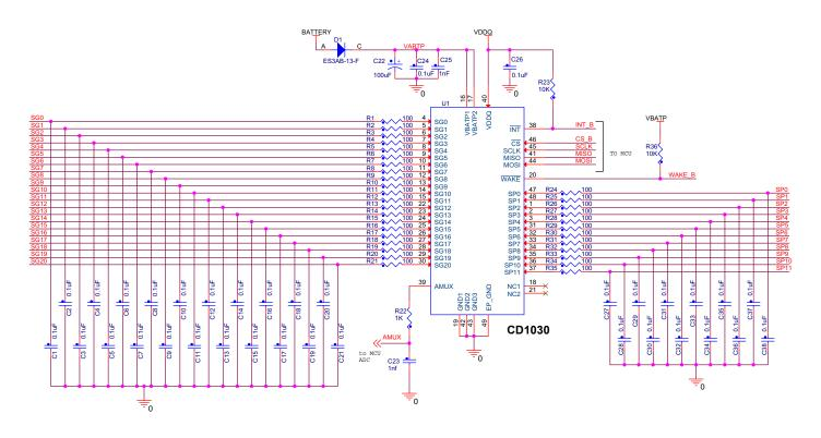
Figure 26. Typical application diagram
