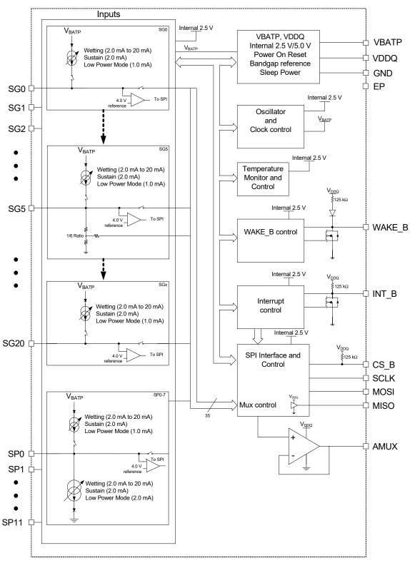
Figure 2. CD1030 internal block diagram
