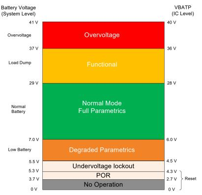
Figure 11. Battery voltage range
