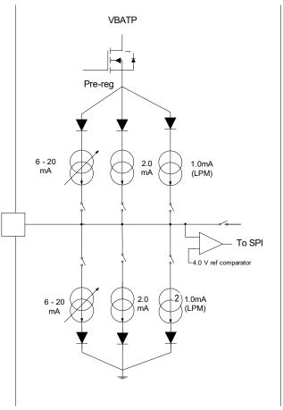
Figure 20. SP block diagram
