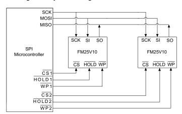
Figure 3. System Configuration with SPI Port
