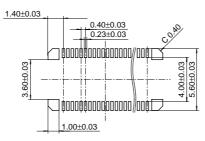
Recommended metal mask pattern Metal mask thickness: Here, 150 μm (Terminal portion opening area ratio: 53 %) (Metal portion opening area ratio: 100 %)
