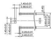
Recommended metal mask pattern Metal mask thickness: Here, 120 μm (Terminal portion opening area ratio: 66 %) (Metal portion opening area ratio: 100 %)
