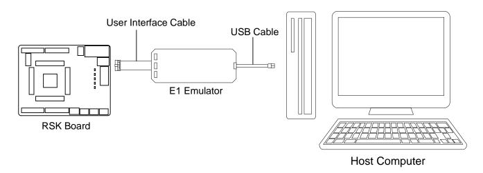
Figure 4-2: Debugger Connection Diagram
