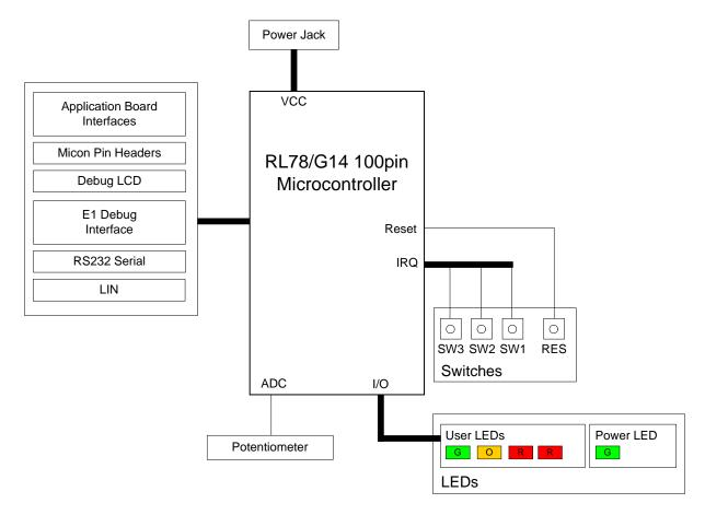
Figure 4-1: Internal Board Block Diagram
