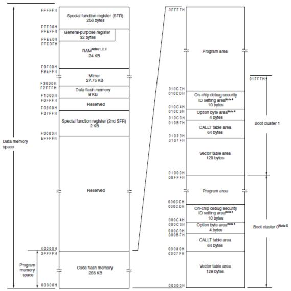
Notes 1. Use of the area F9F00H to FA309H that is used as a work area for the library is prohibited when using the self-programming and data flash functions.
