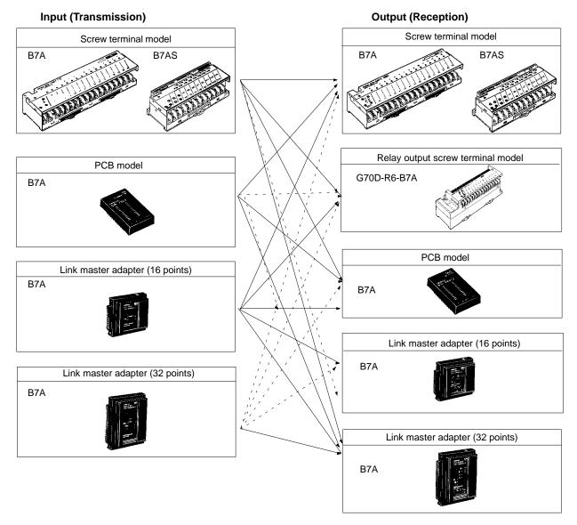
Note: The I/O delay time values of 16-point Link Terminals with Adapters are either 3 ms (typical, for high-speed models) or 19.2 ms (typical, for normal-speed models). Use a combination of an Input and an Output Link Terminal with the same I/O delay time. Connect two 32-point Link Terminals with Adapters together or a 32-point Link Terminal with an Adapter to two 16-point Link Terminals.
