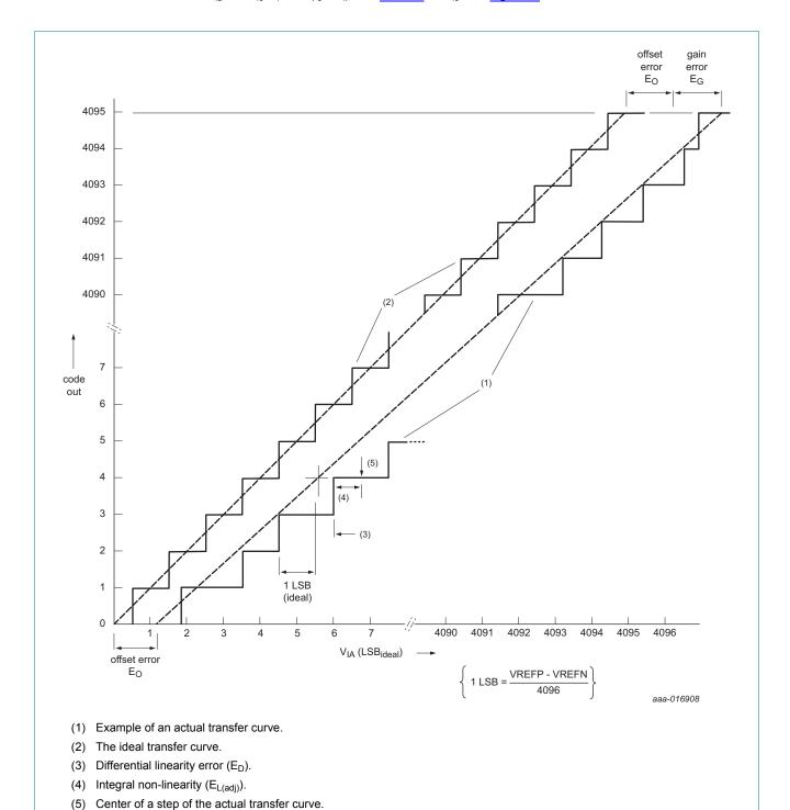
Fig 27. 12-bit ADC characteristics
