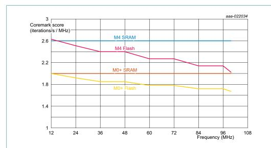
Conditions:  $V_{DD}$  = 3.3 V;  $T_{amb}$  = 25 °C; active mode; all peripherals disabled; BOD disabled; See the FLASHCFG register in the LPC5411x, UM10914 User Manual for system clock flash access time settings. Measured with Keil uVision 5.17. Optimization level 3, optimized for time ON.
