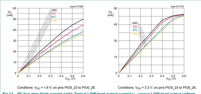
Fig 14. I<sup>2</sup>C-bus pins (high current sink): Typical LOW-level output current I<sub>OL</sub> versus LOW-level output voltage V<sub>OL</sub>
