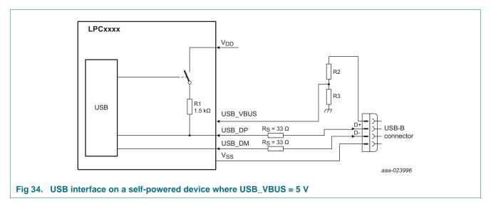
The internal pull-up (1.5 k $\Omega$ ) can be enabled by setting the DCON bit in the DEVCMDSTAT register to prevent the USB from timing out when there is a significant delay between power-up and handling USB traffic. External circuitry is not required.
