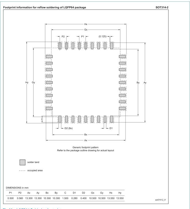
Fig 39. LQFP64 Soldering footprint
