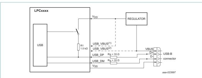
Two options exist for connecting VBUS to the USB\_VBUS pin:
