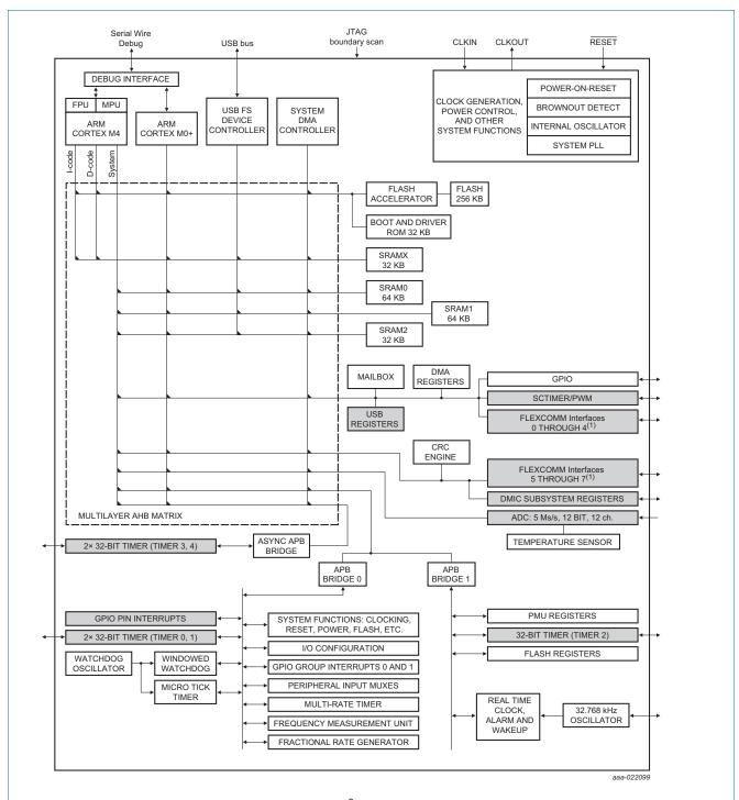
Each Flexcomm Interface includes USART, SPI, and  $I^2C$  functions. Flexcomm Interfaces 6 and 7 each also provide an I2S function. Grey-shaded blocks indicate peripherals that provide DMA requests or are otherwise able to trigger DMA transfers
