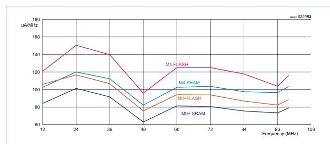
Conditions: VDD = 3.3 V; Tamb = 25 °C; active mode; all peripherals disabled; BOD disabled; Prefetch disabled in FLASHCFG register. See the FLASHCFG register in the LPC5411x, UM10914 User Manual for system clock flash access time settings. SRAM0 and SRAMX powered. SRAM1 and SRAM2 powered down. Measured with Keil uVision 5.17. Optimization level 0, optimized for time OFF.
