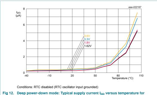
different supply voltages V<sub>DD</sub>
