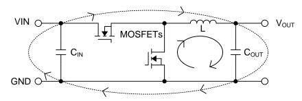
Figure 65. Current Loop of Buck DC/DC Converter
