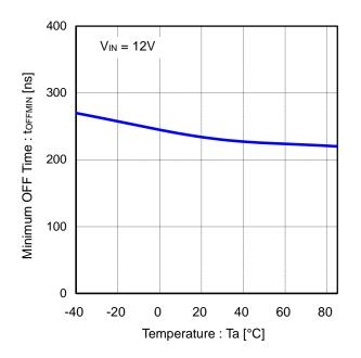
Figure 18. Minimum OFF Time vs Temperature
