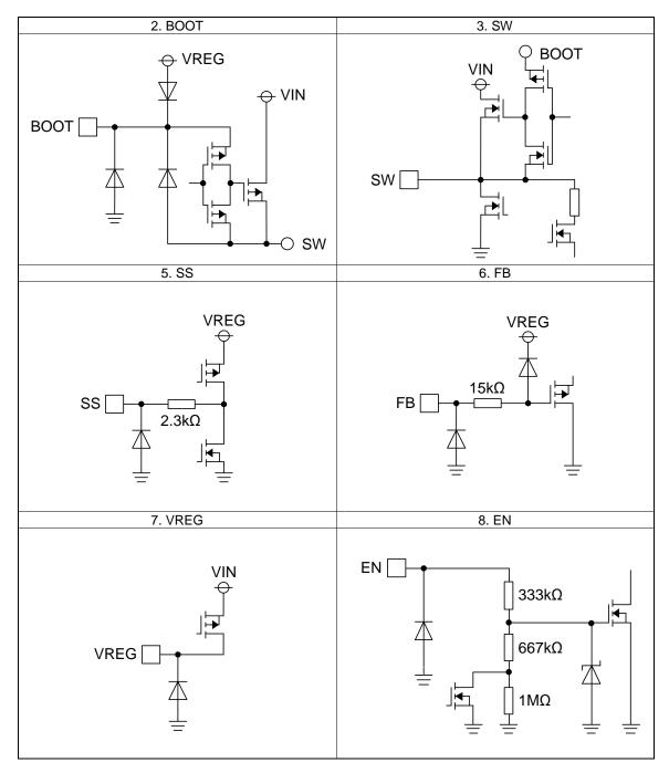
Figure 67. I/O Equivalence Circuits
