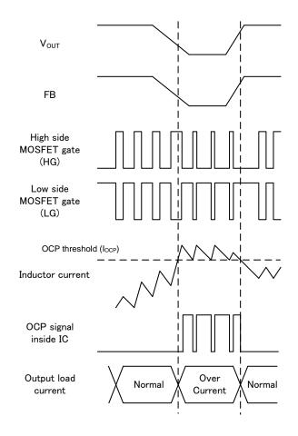
Figure 40. Over Current Protection Timing Chart
