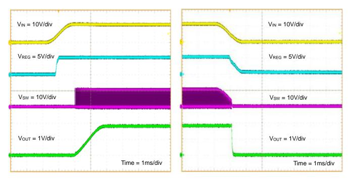
Figure 23. Start-up Waveform (V\_{IN} = V\_{EN}) (V\_{IN} = 12V, V\_{OUT} = 1.8V, I\_{OUT} = 3A, C\_{SS} = 3300 pF)
