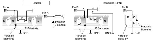
Figure 68. Example of monolithic IC structure
