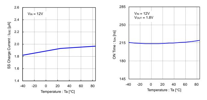
Figure 16. SS Charge Current vs Temperature
