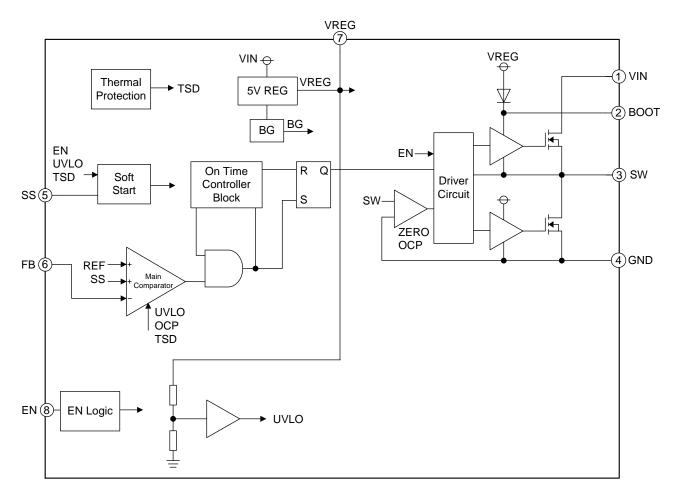
Figure 3. Block Diagram
