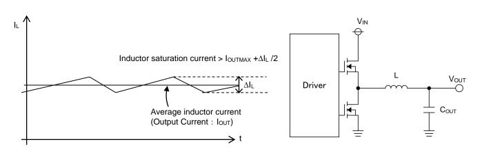
Figure 62. Waveform of Current through Inductor
