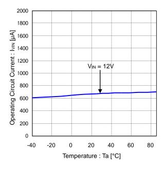
Figure 4. Operating Circuit Current vs Temperature
