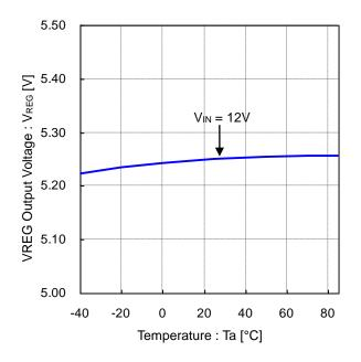
Figure 11. VREG Output Voltage vs Temperature
