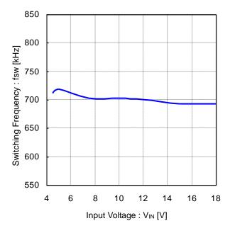
Figure 31. Switching Frequency vs Input Voltage ( $V_{OUT} = 1.8V$ ,  $I_{OUT} = 3A$ ,  $L = 2.2\mu$ H,  $C_{OUT} = 22\mu$ F x 2)
