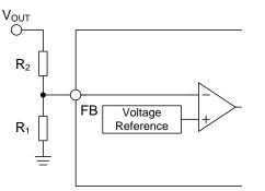
$$V_{OUT} = \frac{R_1 + R_2}{R_1} \times 0.765 ~[V]$$
