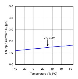
Figure 10. EN Input Current vs Temperature
