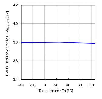
Figure 12. UVLO Threshold Voltage vs Temperature
