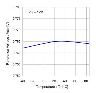
Figure 14. Reference Voltage vs Temperature
