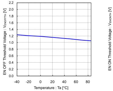
Figure 8. EN OFF Threshold Voltage vs Temperature
