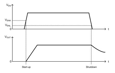
Figure 38. Start-up and Shutdown with Enable
