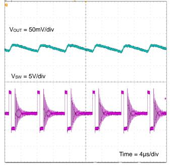
Figure 45. V<sub>OUT</sub> Ripple I<sub>OUT</sub> = 0.1A  $(V_{IN} = 12V, V_{OUT} = 5.0V)$
