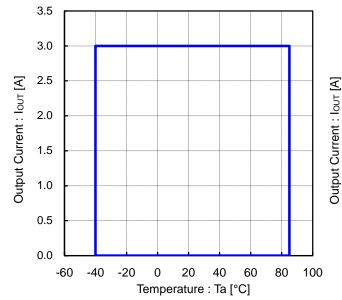
Figure 21. Operational Range  $V_{IN} = 12V$ ,  $V_{OUT} = 1V$  (Tj<150°C) (Measured on FR-4 board 67.5 mm x 67.5 mm, Copper Thickness : Top and Bottom 70µm, 2 Internal Layers 35µm)
