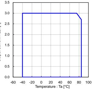
Figure 22. Operational Range  $V_{IN} = 12V$ ,  $V_{OUT} = 5V$  (Tj<150°C) (Measured on FR-4 board 67.5 mm x 67.5 mm, Copper Thickness : Top and Bottom 70µm, 2 Internal Layers 35µm)
