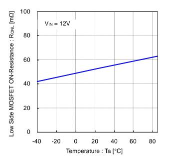
Figure 20. Low Side MOSFET ON-Resistance vs Temperature
