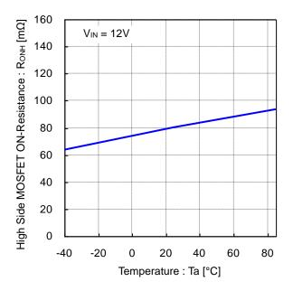
Figure 19. High Side MOSFET ON-Resistance vs Temperature
