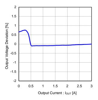
Figure 34. Vout Load Regulation (VIN=12V, Vout=1.8V)
