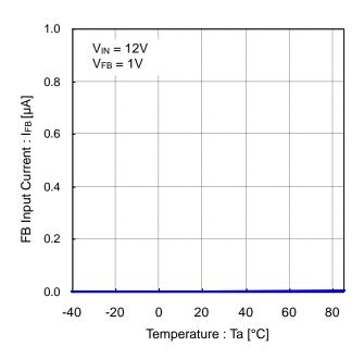
Figure 15. FB Input Current vs Temperature
