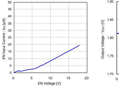
Figure 6. EN Input Current vs EN Voltage
