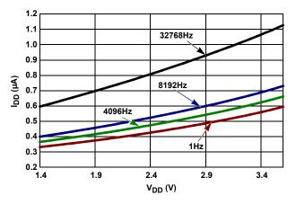
FIGURE 4. I<sub>DD</sub> vs V<sub>DD</sub> vs F<sub>OUT</sub>
