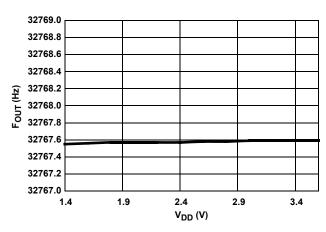
FIGURE 5.  $F_{OUT}$  VS  $V_{DD}$  WITH A TYPICAL 32.768kHZ CRYSTAL
