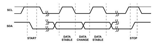
FIGURE 7. VALID DATA CHANGES, START, AND STOP CONDITIONS
