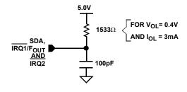
FIGURE 1. STANDARD OUTPUT LOAD FOR TESTING THE DEVICE WITH  $\ensuremath{\text{V}_{DD}} = 5.0\ensuremath{\text{V}}$
