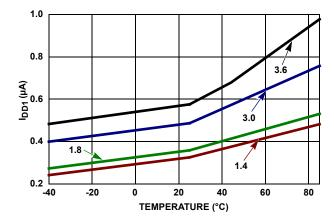
FIGURE 3. I<sub>DD1</sub> vs TEMPERATURE
