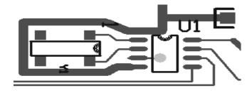
FIGURE 12. SUGGESTED LAYOUT FOR ISL12057 AND CRYSTAL
