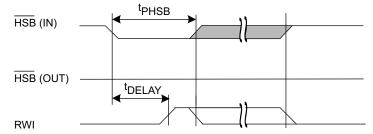
$\overline{\text{HSB}}$  pin is driven  $\underline{\text{HIGH}}$  to  $V_{CC}$  only by Internal 100 K $\Omega$  resistor,  $\overline{\text{HSB}}$  driver is  $\underline{\text{disa}}$ bled SRAM is disabled as long as  $\overline{\text{HSB}}$  (IN) is driven LOW.
