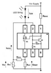
Figure 14 Constant LED Current Temperature Compensation for AL5801
