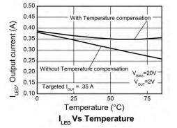
Figure 15 LED Current Variation with and without Temperature Compensation
