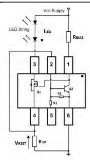
Figure 13 Typical Application Circuit for Linear Mode Current Sink LED Driver
