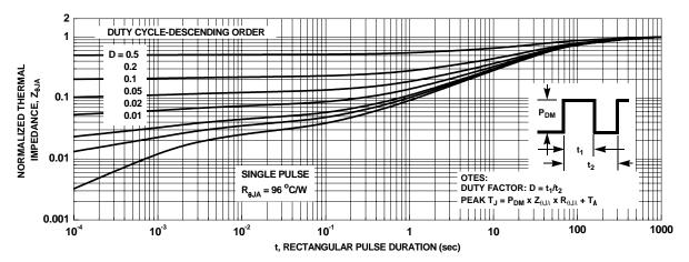
Figure 14. Transient Thermal Response Curve
