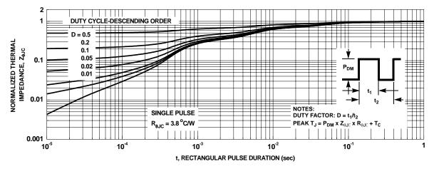
Figure 13. Transient Thermal Response Curve
