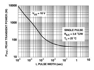
Figure 12. Single Pulse Maximum Power Dissipation
