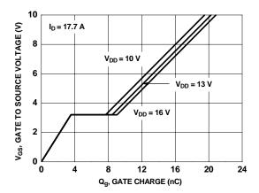
Figure 7. Gate Charge Characteristics
