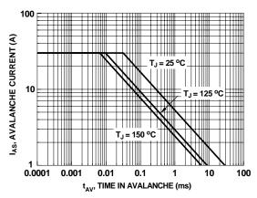
Figure 9. Unclamped Inductive Switching Capability
