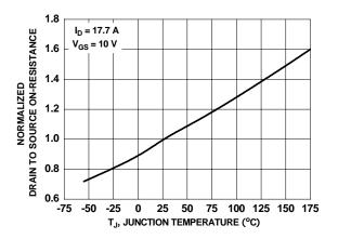
Figure 3. Normalized On-Resistance vs Junction Temperature
