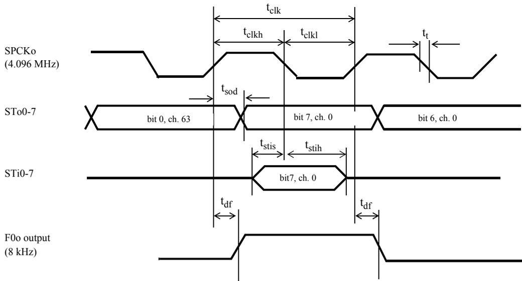
F0 Frame Sync with Positive Polarity (SPFP = 1)
