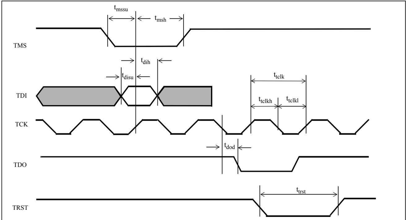
Figure 34 - Boundary Scan Test Port Timing
