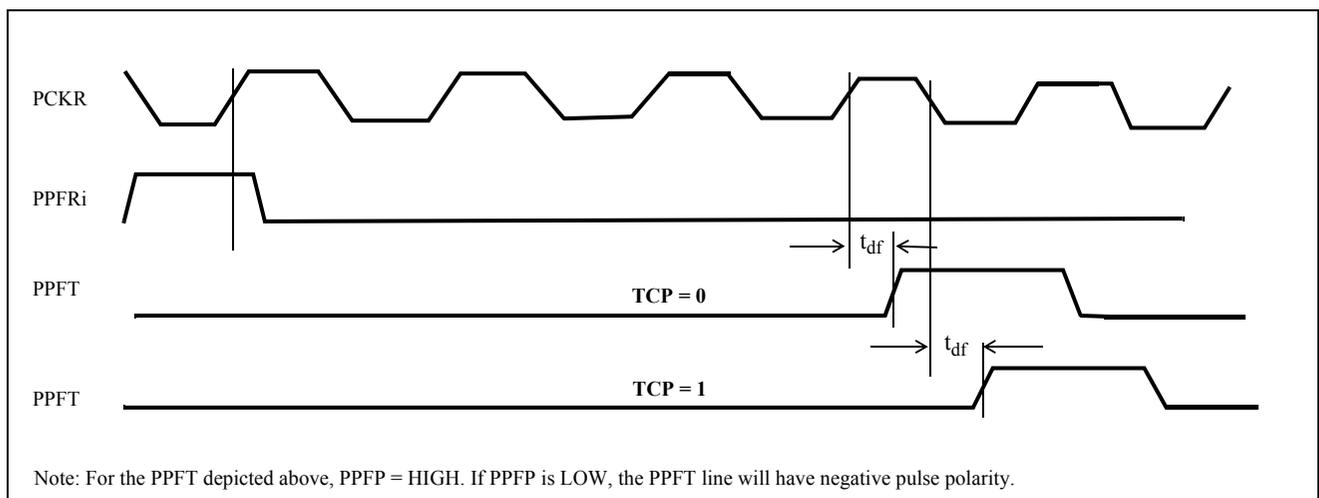
**Figure 29 - Parallel Port in Timing Mode 4**
