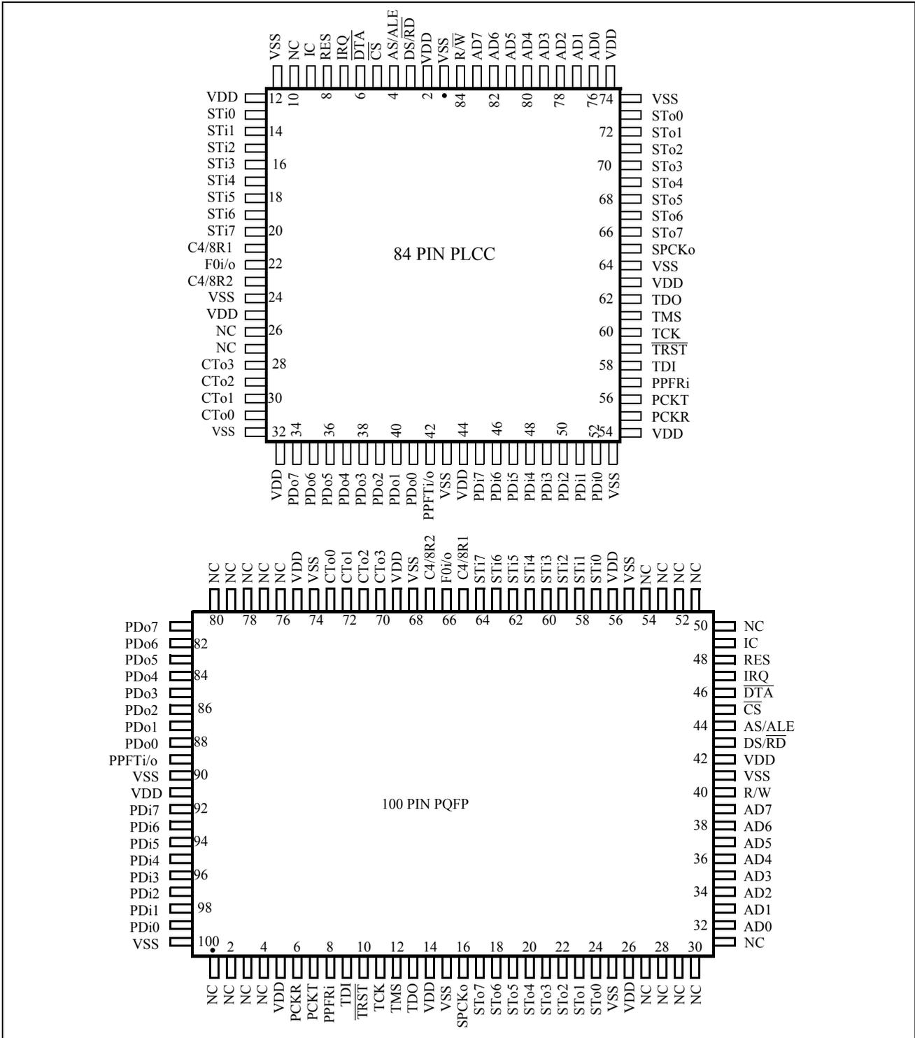
Figure 2 - Pin Connections
