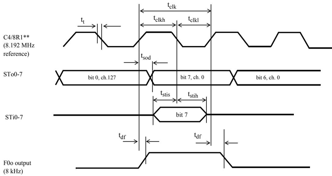
Frame Sync with Positive Polarity (SPFP = 1)
