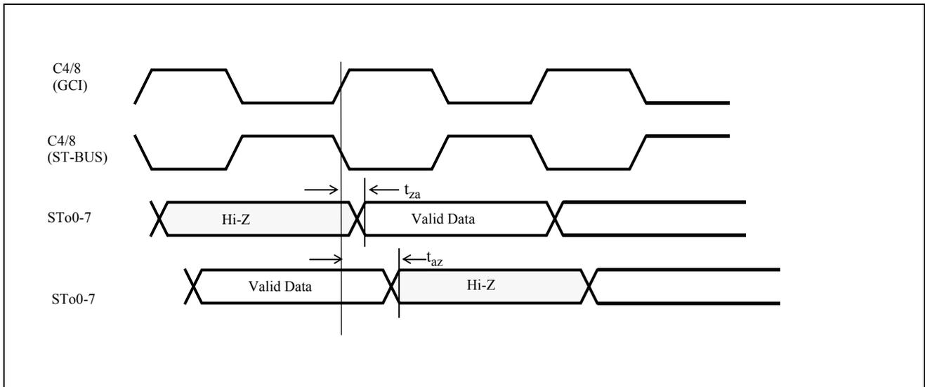
**Figure 23 - Per-Channel Tristate Characteristics at all Data Rates**
