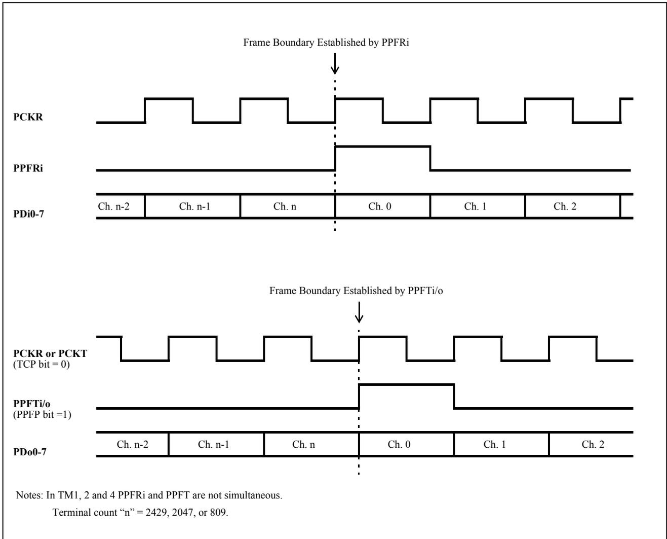
**Figure 4 - Parallel Data Port Functional Timing**
