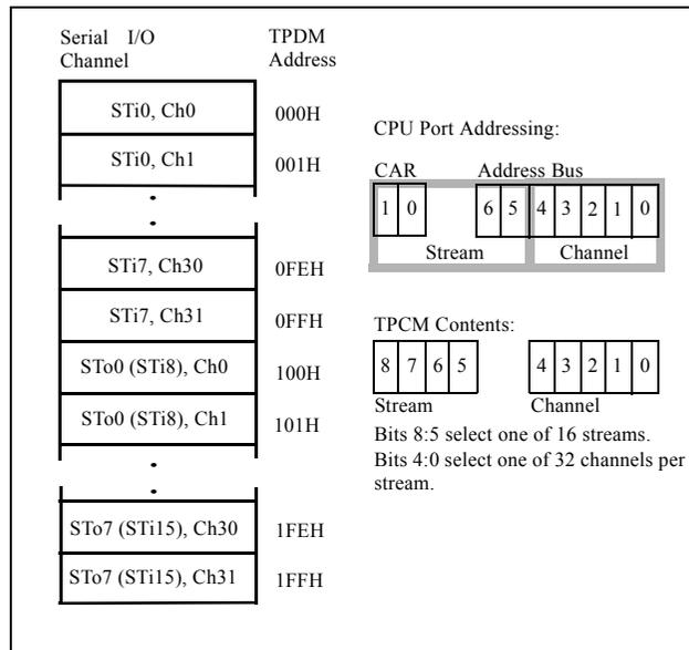
**Figure 12a - 2.048 Mbps Add/Drop Mode TPDM Addressing**
