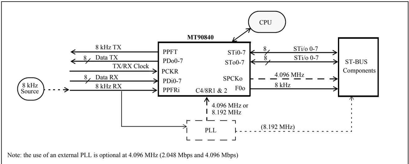
Note: the use of an external PLL is optional at 4.096 MHz (2.048 Mbps and 4.096 Mbps)
