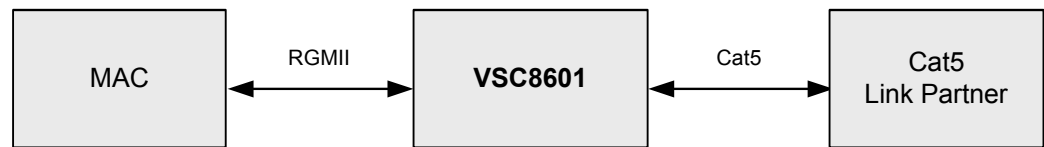
Figure 3. RGMII to Cat5 Block Diagram
