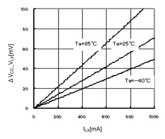
Figure 14. High Side FET ON-Resistance Temperature Characteristics
