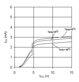
Figure 5. Circuit Current vs  $V_{\text{CC}}$
