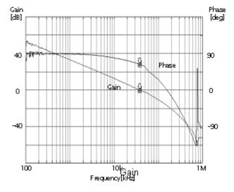
Figure 21. Frequency Response Characteristics (I<sub>O</sub>=3.0A)
