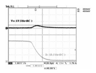
Figure 23. Load Response Characteristics  $(I_0=3A \text{ to } 0A)$
