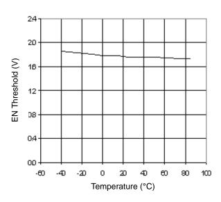
Figure 17. EN Threshold Voltage vs Temperature
