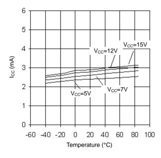
Figure 6. Circuit Current vs Temperature
