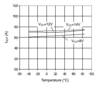
Figure 16. OCP Detect Current vs Temperature
