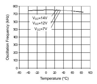
Figure 8. Oscillation Frequency vs Temperature
