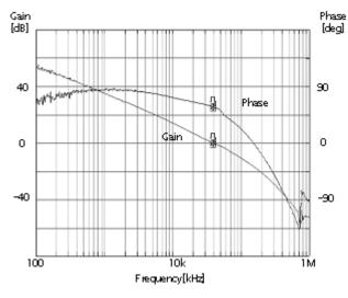
Figure 20. Frequency Response Characteristics (I<sub>O</sub>=1.5A)
