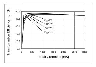
Figure 19. Electric Power Conversion Rate
