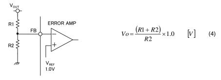
Figure 28. How to Set Feedback Resistors
