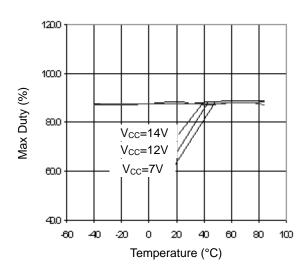
Figure 9. Maximum Duty Cycle vs Temperature
