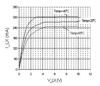
Figure 15. Low Side ON-Resistance Temperature Characteristics
