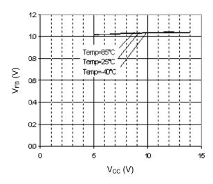
Figure 11. FB Threshold Voltage vs V<sub>CC</sub>
