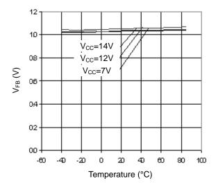
Figure 10. FB Threshold Voltage vs Temperature
