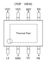
Figure 2. Pin Configuration
