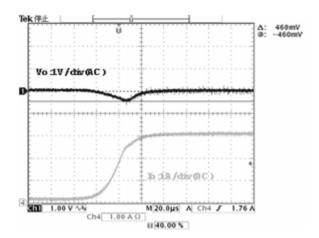
Figure 22. Load Response Characteristics ( $I_0$ =0A to 3A)
