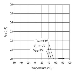
Figure 4. Standby Circuit Current vs Temperature
