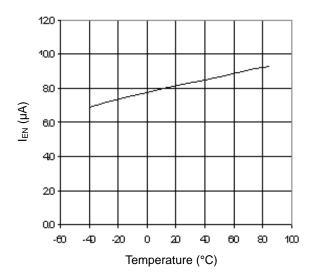
Figure 18. EN Pin Input Current vs Temperature
