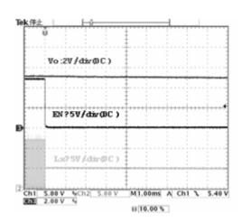
Figure 25. Stop Waveform
