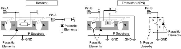
Figure 29. Example of monolithic IC structure
