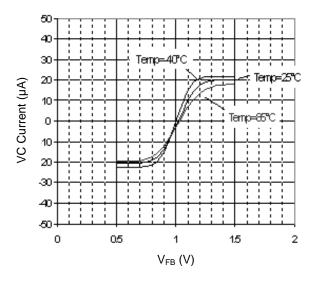
Figure 12. VC Current vs FB Voltage
