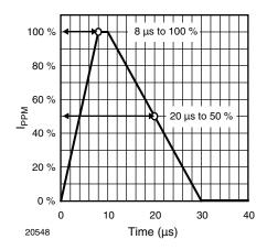
Fig. 2 - 8/20 µs Peak Pulse Current Wave Form acc. IEC 61000-4-5
