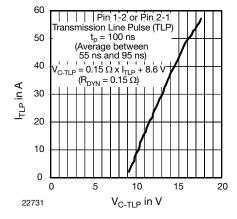
Fig. 8 - Typical Clamping Voltage at 100 ns Transmission Line Pulse
