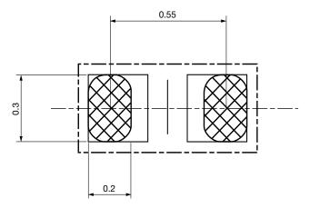
Fig. 2 - Maximum Stencil Openings - for a Stencil Thickness of 80 µm
