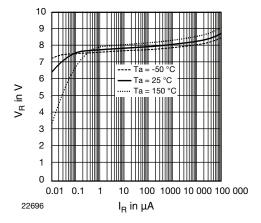
Fig. 4 - Typical Reverse Voltage V<sub>R</sub> vs. Reverse Current I<sub>R</sub>
