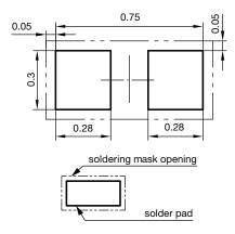
Fig. 1 - Recommended Soldering Pad Design
