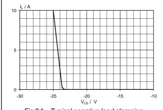
Fig.24. Typical negative load clamping.  $I_L = f(V_{LG})$ ; conditions  $V_{IG} = 0V$ ,  $T_j = 25$ °C
