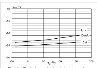
Fig.25. Typical negative load clamping voltage.  $V_{LG} = f(T_i)$ ; parameter  $I_L$ ; condition  $V_{IG} = 0$ V
