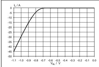
Fig.26. Typical reverse diode characteristic.  $I_L = f(V_{BL})$ ; conditions  $V_{IG} = 0$  V,  $T_j = 25$  °C
