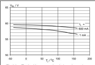
Fig.23. Typical battery to load clamping voltage.  $V_{BL} = f(T_j)$ ; parameter  $I_L$ ; condition  $I_G = 10 \text{mA}$
