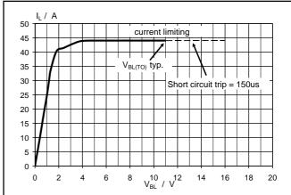
Fig.27. Typical overload characteristic,  $T_{mb} = 25$  °C.  $I_L = f(V_{BL})$ ; condition  $V_{BG} = 16$  V; parameter  $t_p$
