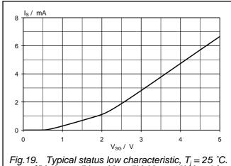
Fig.19. Typical status low characteristic,  $T_i = 25$  °C.  $I_S = f(V_{SG})$ ; conditions  $V_{IG} = 5V$ ,  $V_{BG} = 13V$ ,  $I_L = 0A$
