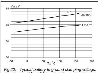
Fig.22. Typical battery to ground clamping voltage.  $V_{BG} = f(T_j)$ ; parameter  $I_G$
