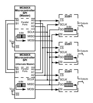
Figure 16. Multiple MCU SPI Control
