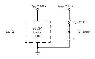
C<sub>1</sub> represents the total capacitance of the test fixture and probe.
