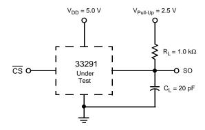
C<sub>L</sub> represents the total capacitance of the test fixture and probe.
