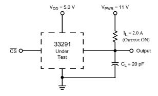
$\ensuremath{C_L}$  represents the total capacitance of the test fixture and probe.
