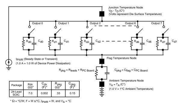
Figure 22. Thermal Model (Electrical Equivalent)
