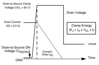
Figure 21. Output Voltage Clamping
