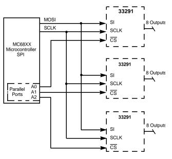
Figure 15. Parallel Input SPI Control
