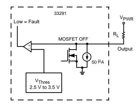
Figure 19. Output OFF Open Load Fault
