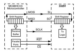
Figure 13. SPI Interface with Microcontroller
