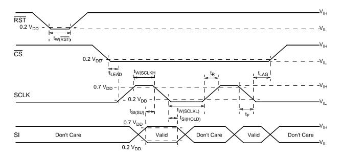
**Figure 4. Input Timing Switch Characteristics**
