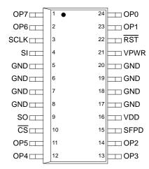
Figure 3. 33291 Pin Connections
