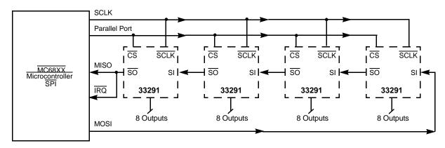
Figure 14. 33291 SPI System Daisy Chain
