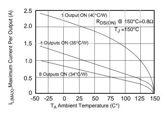
Figure 23. Maximum SOIC Package Steady State Output Current vs. Ambient Temperature
