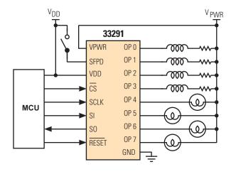
Figure 1. 33291 Simplified Application Schematic
