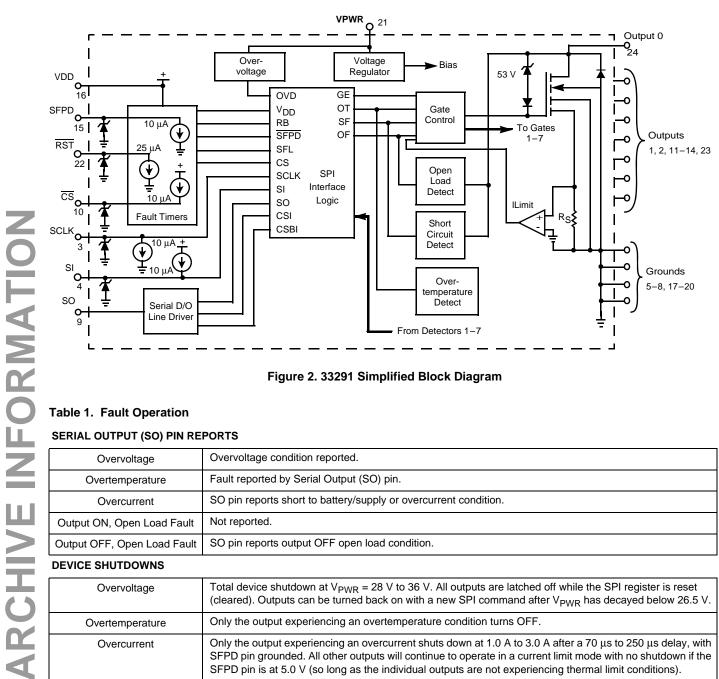
Figure 2. 33291 Simplified Block Diagram
